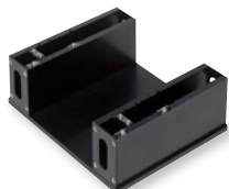
Long-Path Rectangular Cell Holder (P/N 204-23118-01)
